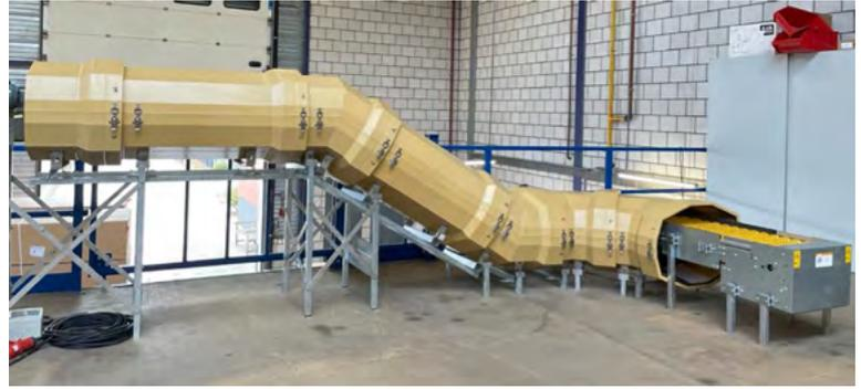
Cover for the transportation of eggs manufactured by TPI Polytechniek B.V.
